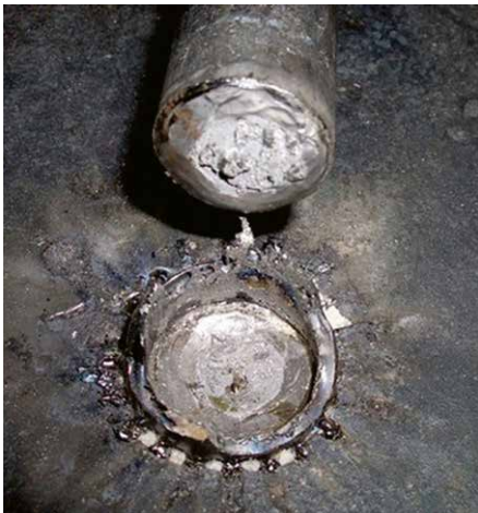
Fig. 17: Failure of the bend test in spite of passing the visual check (© Trillmich)
