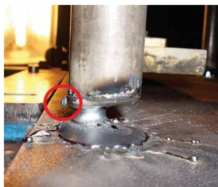
Fig. 5: Slanted melt with plunge impediment (© Trillmich)
