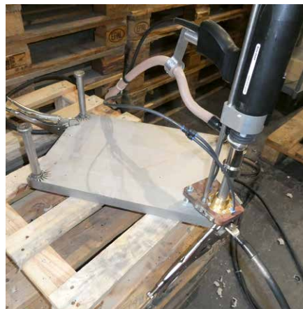
Fig. 14: Successful compensation only with two ground clamps (© Trillmich)
