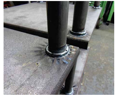
Fig. 9: Flawless result even on the corner of a plate (© Trillmich)
