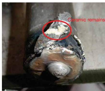
Fig. 6: Splashes caused by a blowing effect prevent the plunge. (© Trillmich)
