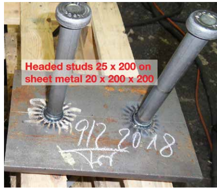
Fig. 8: Flawless result on small anchor plate (© Trillmich)
