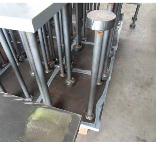
Fig. 1: Anchor bolts, produced from individual parts and welded on manually (© Trillmich)
