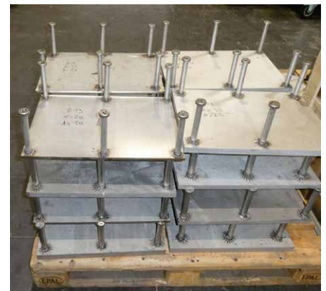
Fig. 12: Stainless steel anchor plates for the nuclear sector (© Trillmich)
